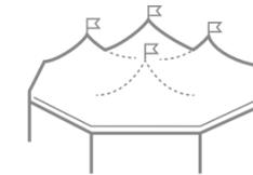
A unique and singular solution, with Meeting we manage to create a single interconnected space without separations or central columns. The internal tubular supporting structure emphasises the design of the roof covering sheet. From an external point of view, it becomes a free and dynamic surface. The largest side of the octagonal structure is 6 meters.
